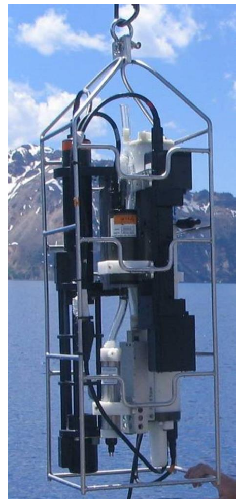
CTD package that measures physical and biological parameters throughout the Crater Lake water column. Tall black sensors on left and right are transmissometers (NPS photo).
