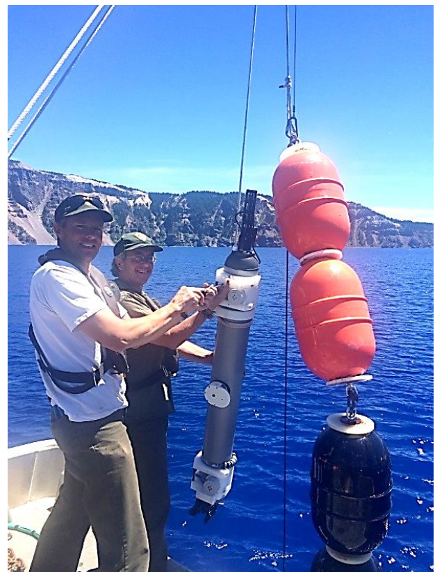
Recovering the ITP instrument from its 580 m long wire mooring line after spending an entire year in Crater Lake (NPS photo).
