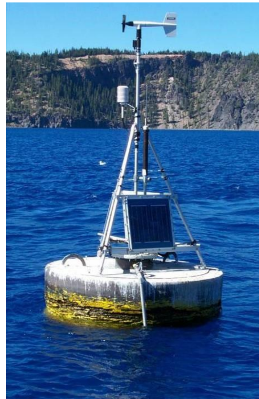
Automated weather station attached to a buoy on Crater Lake. The sensor used for tracking surface water temperature is located under the buoy at a depth of approximately 1 meter (NPS photo).
