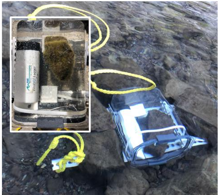
Productivity of attached algae was measured over several days by placing a rock in an acrylic chamber and measuring dissolved oxygen changes with an optical sensor. Inset shows a closeup of the rock and oxygen sensor.
