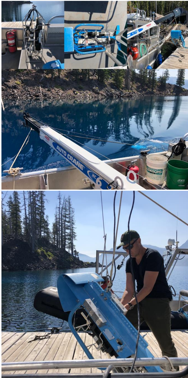
Equipment and setup of CTD sensors for a near shore tow along the shoreline of Crater Lake.
